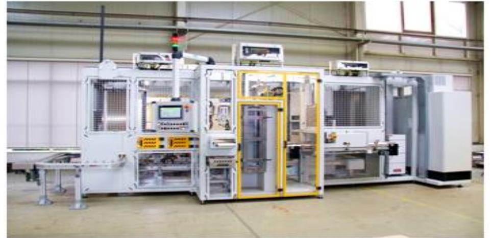
Leak testing devices
