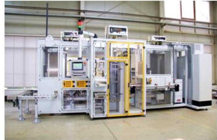
Leak testing devices
