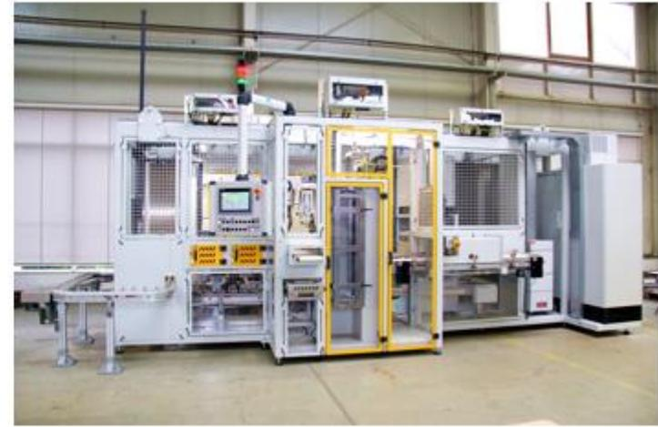
Leak testing devices
